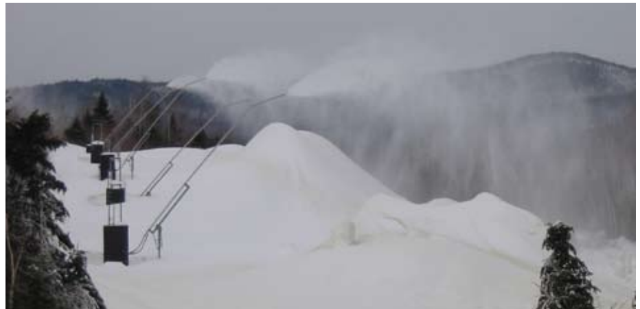
Sewage treatment for the town of Rangeley has evolved quite a ways from the 1960's when treated wastewater was discharged directly into Haley Pond. The new plant, built in 1996, has no direct discharge, instead the treated wastewater is used to create snow.
